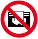
**Do not cover. Warning:** In order to avoid overheating of the appliance, the heater may not be covered over. Never cover the infrared heater with washing or similar items. This can cause a build-up of heat.
